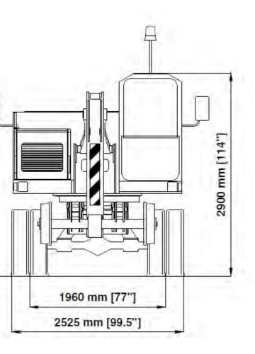
Rail mode – Level rail - Tool pin – unlocked - 0° - height 3m – Distance 5m = 10.97t
