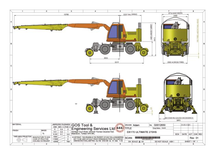
Hydrostatic Drive - DX Ultimate 270HS with 5.5m Dipper and self levelling function (SL)
