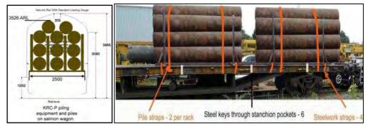
Figure 52: Securing and transportation of pile foundations
