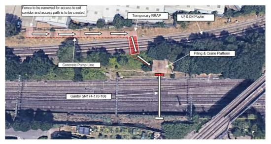
Figure 103: Proposed access route for piling
