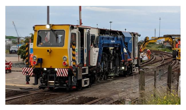
A Volker Rail lightweight tamper is seen on a level crossing at Newhaven Harbour during engineering work at Newhaven Marine aggregate sidings.
