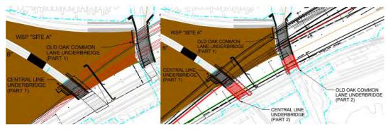
Figure 116: Two phase construction of OOCL and Central Line Underbridge
