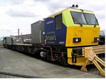
Railtrack MPV, nos. DR98917+DR98967, at Doncaster Works on 27 July 2003. These purpose-built departmental vehicles were built to replace older trains converted from former passenger vehicles.
