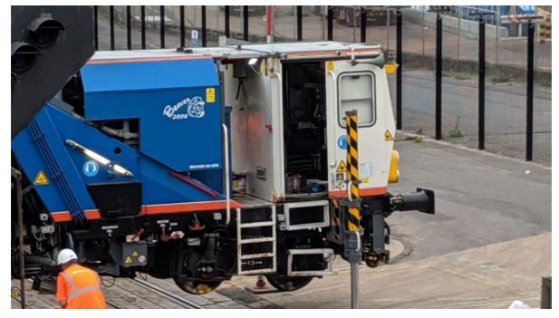
Arms beside each cab on each side stablise the tamper whilst it is lifted off the ground. The arms at each end lift the machine.
