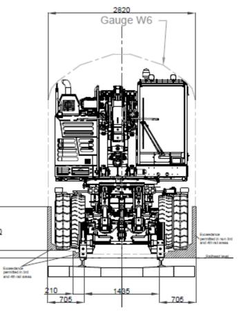
Rail mode – Level rail - Tool pin – unlocked - 0° - height 3m – Distance 5m = 10.97t
