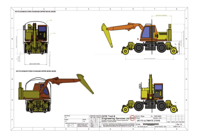
Hydrostatic Drive - DX Ultimate 270HS with 2.1m Dipper
