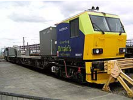
Railtrack MPV, nos. DR98917+DR98967, at Doncaster Works on 27 July 2003. These purpose-built departmental vehicles were built to replace older trains converted from former passenger vehicles.
