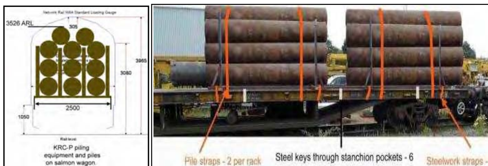
Figure 52: Securing and transportation of pile foundations
