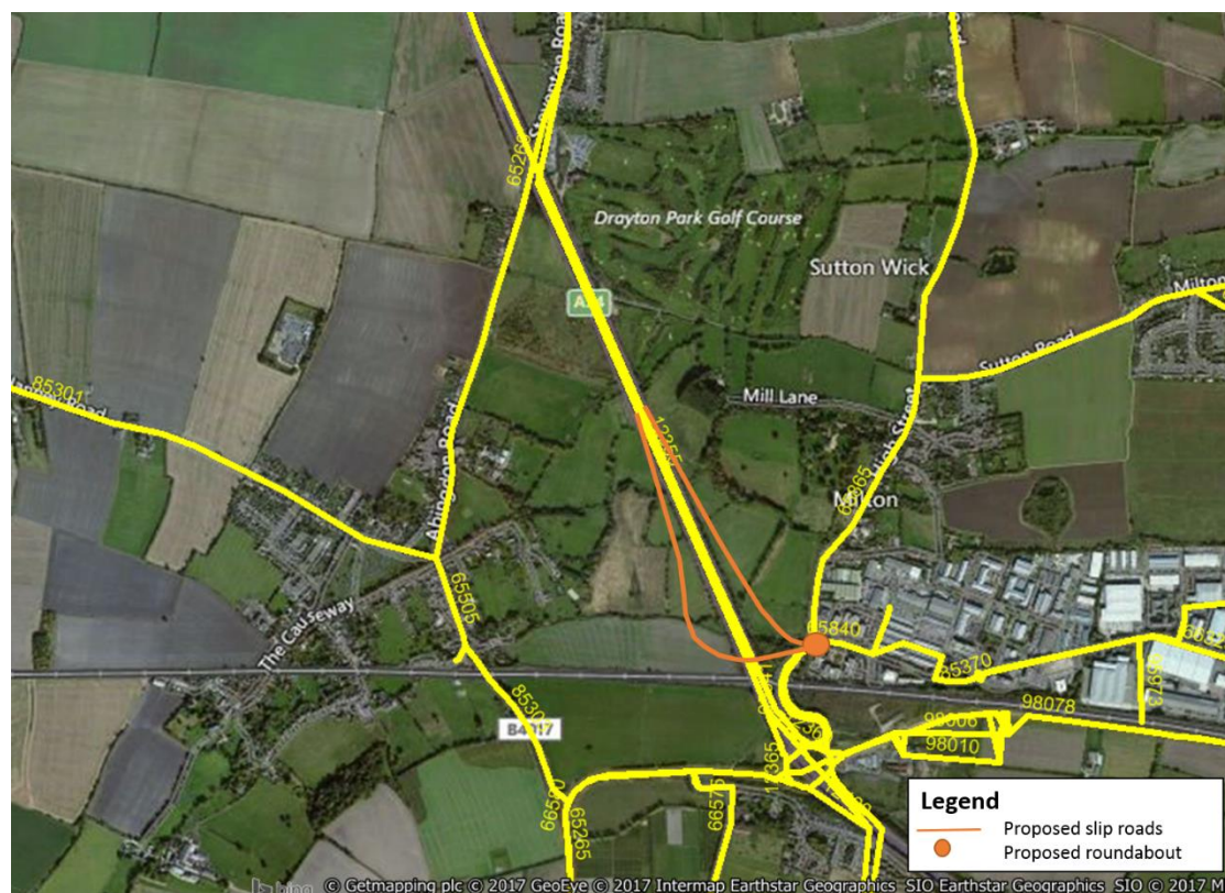
Figure 19 Proposed slip roads and roundabout
