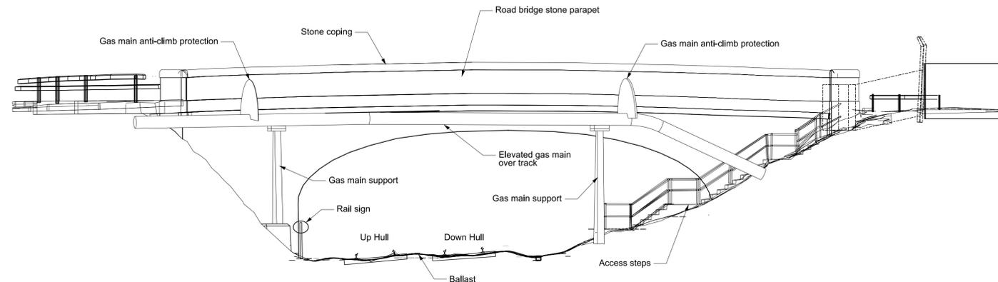
Elevation B-B Existing: Road Bridge East Elevation
