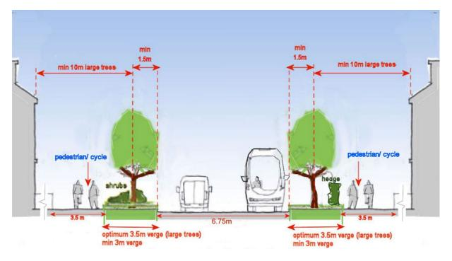
Figure 34: Example Cross Section of a Connector Street
