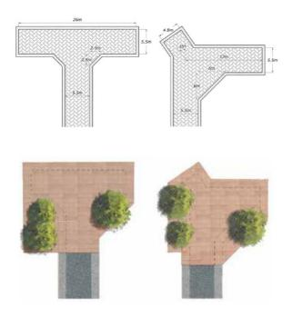
Figure 26: Alternative Refuse Collection Vehicle Turning Heads
