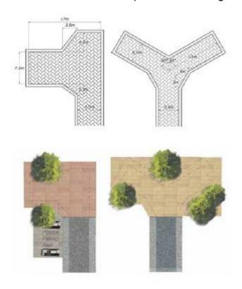
Figure 25: Standard Refuse Collection Vehicle Turning Heads
