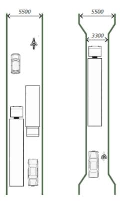
Figure 15: Minimum Carriageway Widths (various locations)
