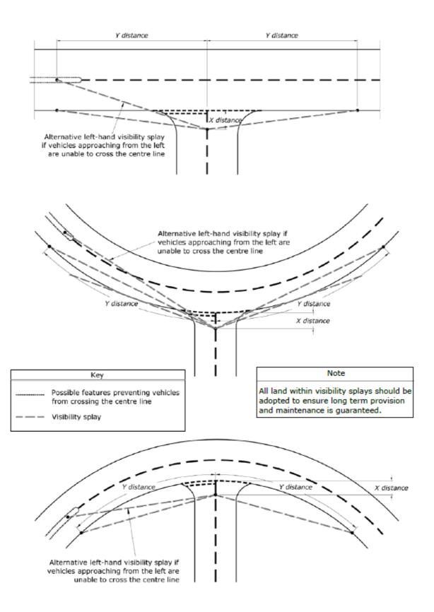
Figure 18: Diagrams Displaying the Different Measurement of Splays
