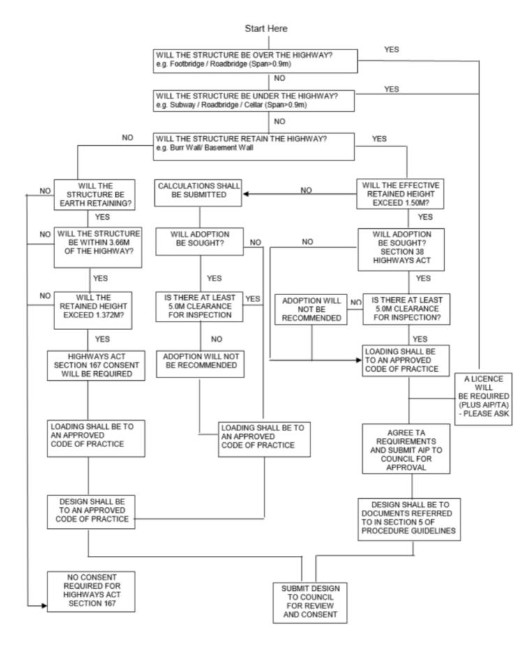
Figure 56: Structures affecting the Highway for which Consent is Required
