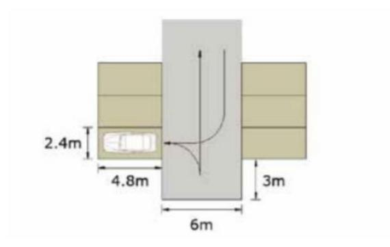
Figure 42: Car Parking Aisle Dimensions
