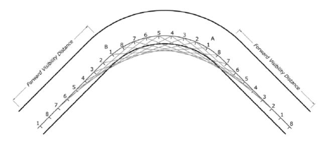
Figure 21: Measuring Forward Visibility Envelope
