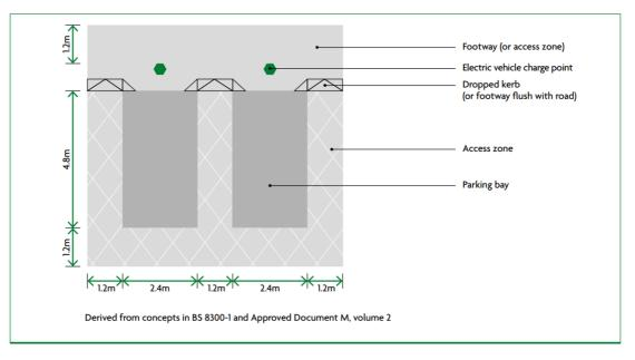
Figure 44: Suggested Accessible Charge Point Layout
