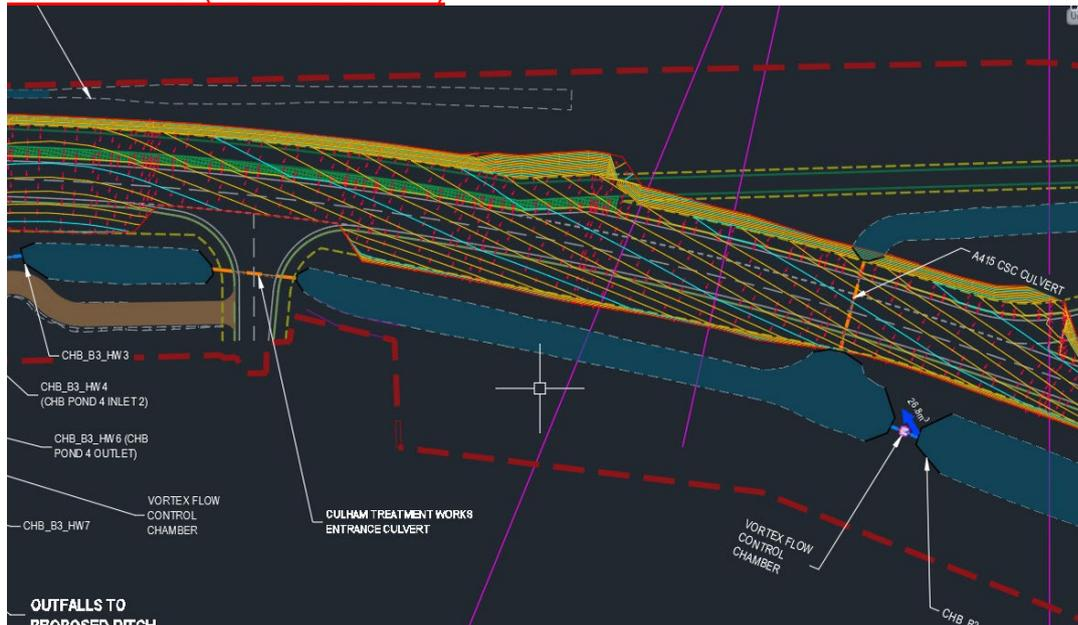
As per OCC requirement over the edge drainage has been used to collect the runoff from road between 985 and 1690 using SuDS.
